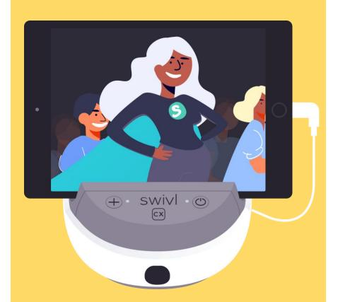
The NEW Swivl CX robot rotates to follow the teacher automatically. It connects to multiple Markers for audio throughout the room and uses the tethered iPad (or mobile device) for recording video or streaming (Zoom, MS Teams, Google Meets). Its easy for teachers to set up and operate as a daily part of class.
